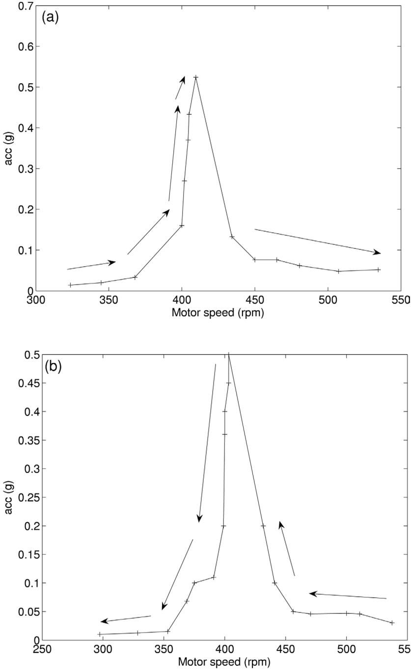
Figure 5. System response vs. motor speed: (a) increasing frequency and (b) decreasing frequency.
