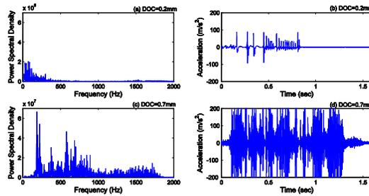
Fig. 4. Power spectral density and time traces of the tool acceleration for (a, b) DOC=0.20mm, (c, d) DOC=0.70mm and 12 strokes/min cutting speed.
