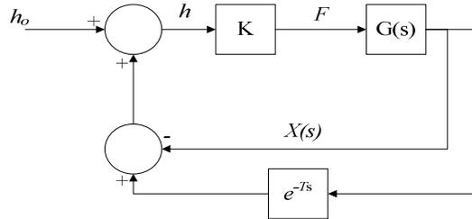
Figure 9: Closed-loop representation of regenerative chatter
