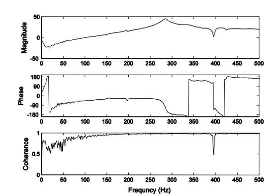
Figure 3: Frequency response function for the tool (magnitude, phase and coherence).
