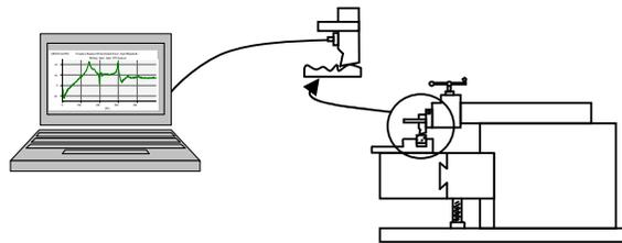
Figure 2: Shaper machine, workpiece, and data acquisition system layout.
