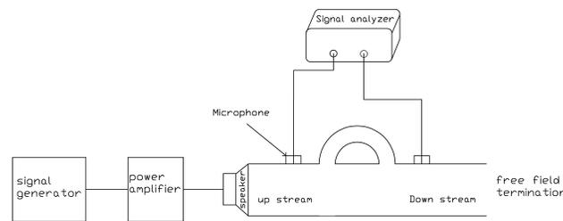
Figure 8. Experimental setup to verify numerical analysis
