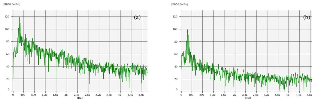
Figure 9: SPL (a) before and, (b) after HQ tube of the PVC pipe setup
