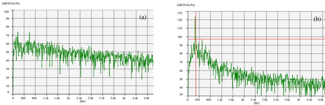
Figure 6. SPL (a) without combustion, (b) with combustion
