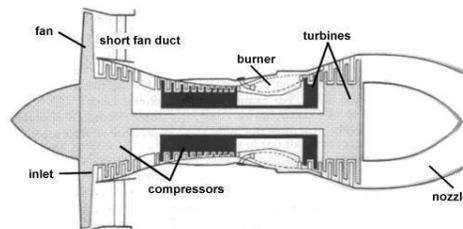
Figure 2. High-Bypass Turbofan [6]
