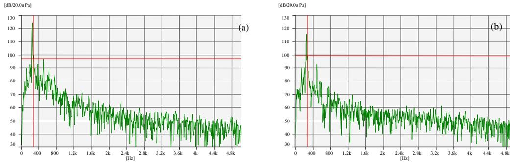
Figure 10: SPL (a) before and, (b) after HQ tube of the test rig
