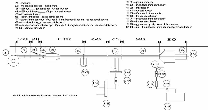
Figure 5. Schematic diagram of the burner-combustor system.
