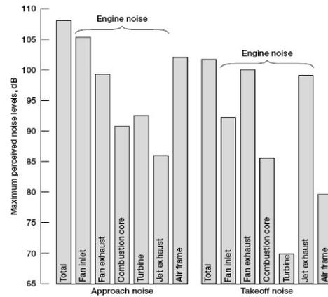
Figure 1. A breakdown of the noise components of a typical engine [1]
