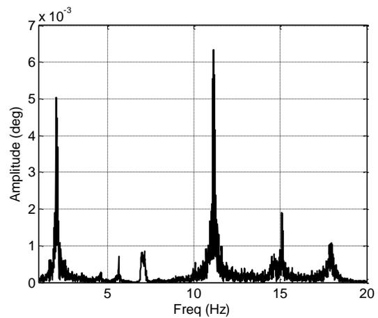
Figure 12. Blade Torsional deformation spectrum
