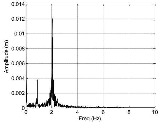
Figure 11. Blade flapwise deformation spectrum
