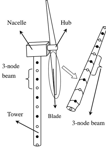
Figure 1. Structure model of wind turbine
