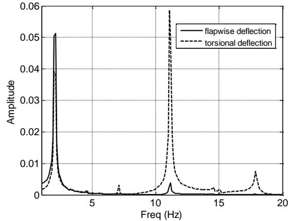
Figure 3. Blade flapwise and torsional deformation spectrum
