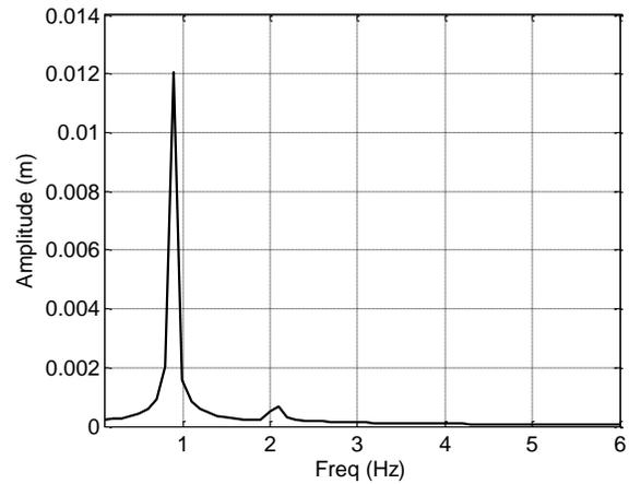
Figure 4. Tower fore-aft deformation spectrum
