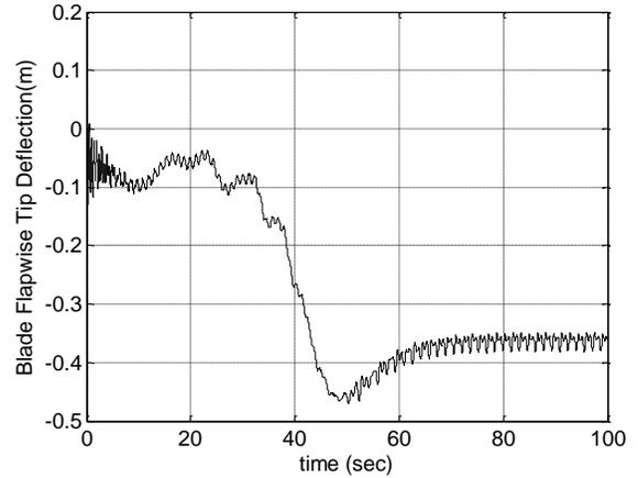
Figure 7. Blade flapwise deformation
