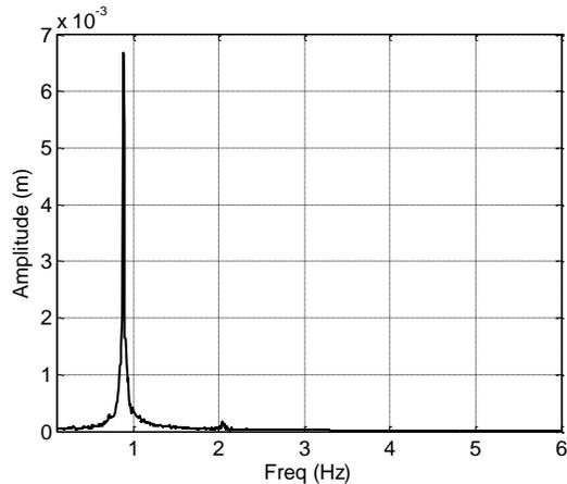
Figure 13. Tower fore-aft deflection spectrum
