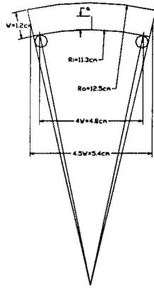
Figure 2 Three point bending specimen cut from the pipe wall for testing
