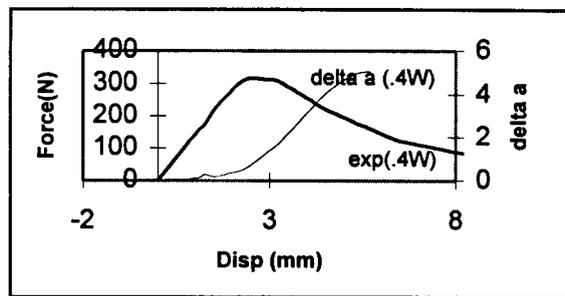
Figure 11 Prediction of the crack growth behavior of the bending specimen
