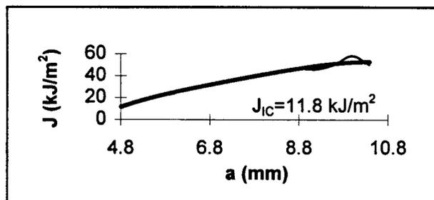
Figure 12 Single specimen J-R curve for the bending specimen, obtained by the key curve method
