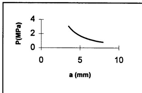
Figure 16 Critical pressure vs. crack length for the pipe
