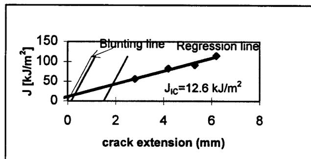
Figure 4 J-Resistance curve for PVC at 25 cm/min
