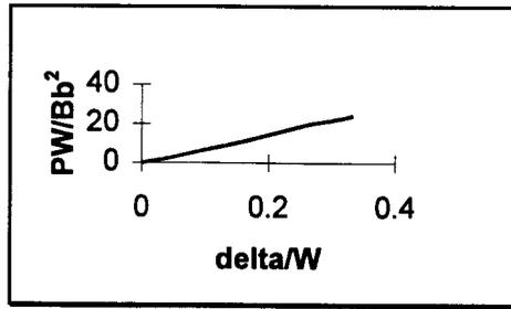
Figure 8 Normalized P-Δ curve from finite element calculations
