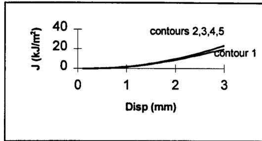
Figure 6 J-integral computed in different contours [a=0.5W]
