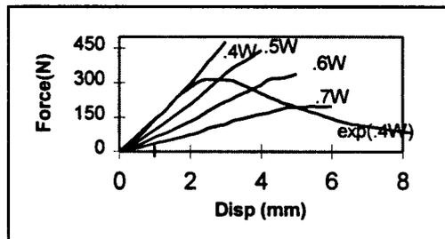
Figure 7 Load-Displacement curves for different crack to width ratios (Finite Element Results)
