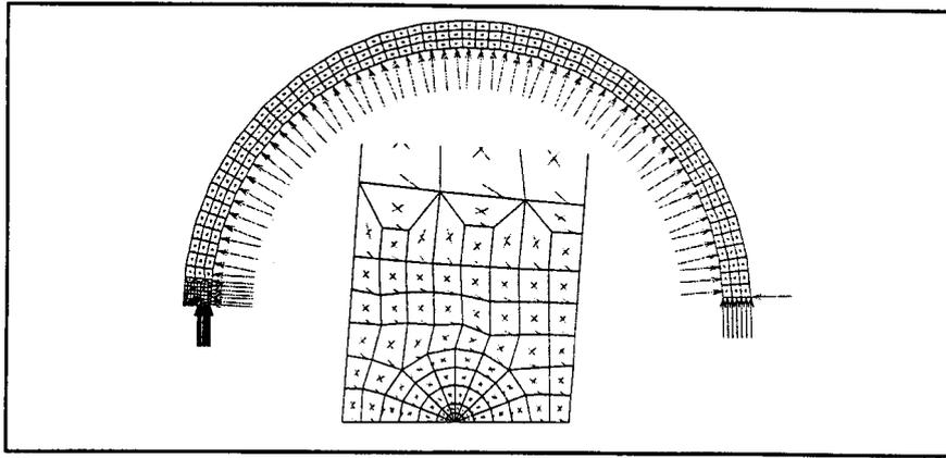
Figure 14 Finite element mesh of the half pipe model
