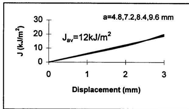
Figure 3 J-integral vs. load-point displacement for PVC at 25 cm/min
