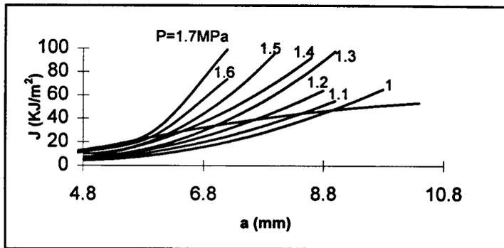
Figure 15 A J-integral crack driving force diagram for the pipe
