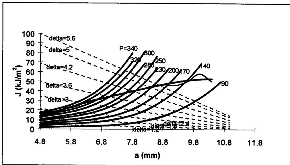
Figure 13 A  $J$ -integral crack driving force diagram for the bending specimen
