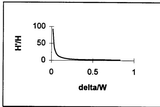
Figure 9 Finite element key curve function for the bending specimen
