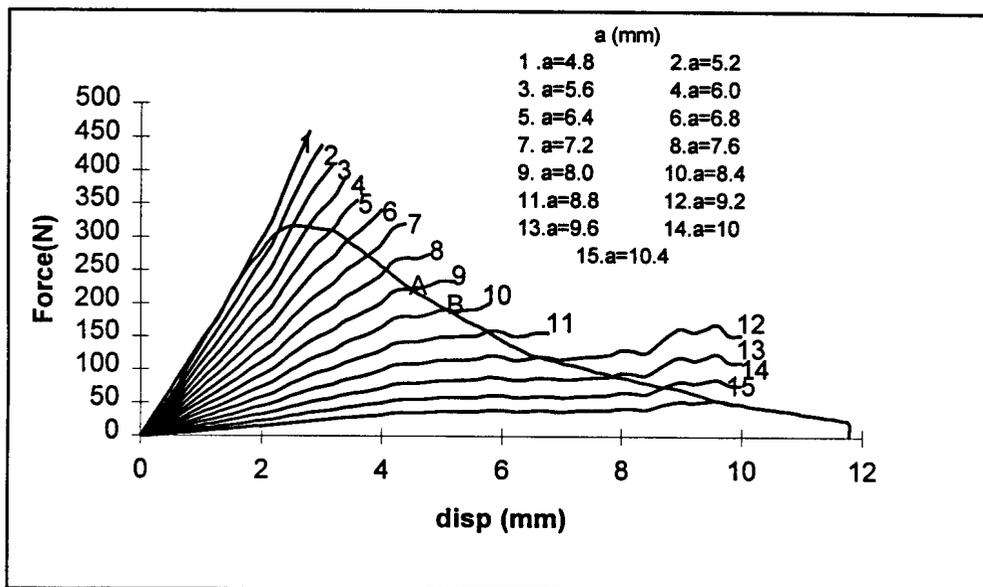
Figure 10 Generated load-displacement curves for different crack lengths
