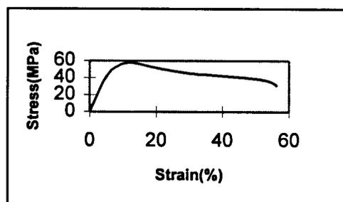
Figure 1 Actual stress-strain diagram for PVC at 250 mm/min
