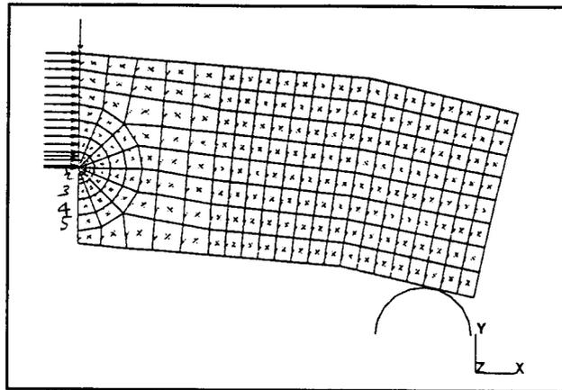
Figure 5 Finite element mesh ( $a=0.4W$ )
