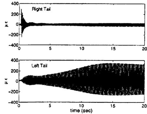
Figure 7: Energy transfer through the mechanism of one-to-one autoparametric resonance
