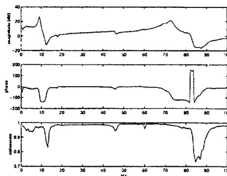
Figure 4: Frequency-response and coherence functions for the left tail
