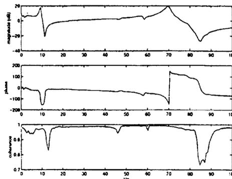
Figure 3: Frequency-response and coherence functions for the right tail
