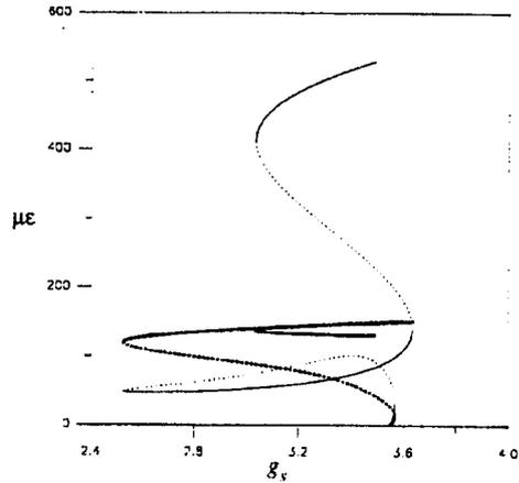
Figure 10: Theoretically obtained amplitude-response curve at 18.0 Hz when  $k = 87$  ( $1/sec^2$ )
