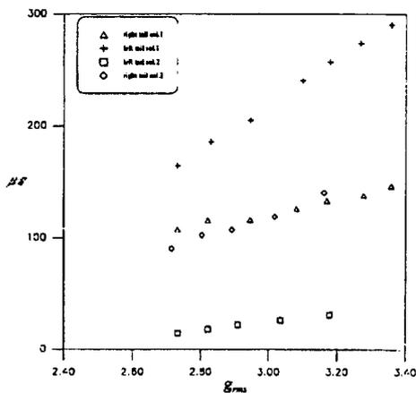
Figure 9: Experimentally obtained amplitude-response curves (left tail response is larger than that of right tail) at 18.0 Hz. (Forward Sweep)
